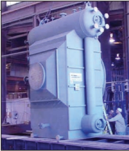
FIGURE 2. A cross-flow boiler with finned tubes (left) is very compact, while a longitudinal gas boiler with plain tubes (right) has a large footprint
