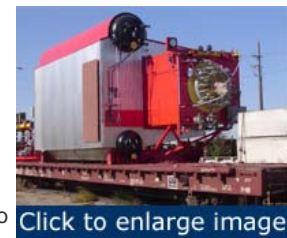
Figure 1. Typical D-type package boiler is ready to be installed.
